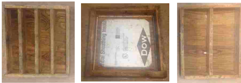
Figure 3.8: Formwork for Durability Specimens.
