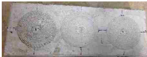
Figure 3.25: 35% 28d Abrasion Specimen post test
