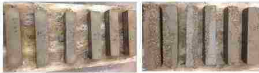
Figure 3.27: 60T Freeze-Thaw Specimens (Left: Before, Right: After)
