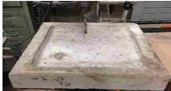
Figure 3.26: 35% 90d Chloride Ion Penetration Specimen
