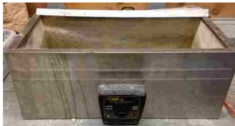
Figure 3.11: Hot Temperature Water Bath tank
